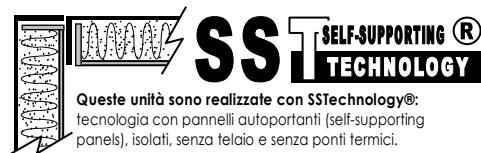
These units are realised with SSTTechnology®: technology with self-supporting panels, insulated, without frame and without thermal bridges.
